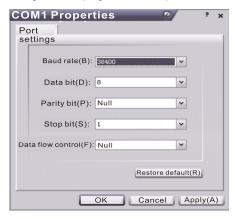
Change the serial port configuration to 38400-baud rate, 8 data bits, no parity bit, 1 stop bit, no data flow control, press the "OK" button, you have set up the Windows serial port Hyper Terminal.
