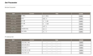
The Item and Items columns list the parameters that can be changed, the Current column lists the present parameter values, the New column can select or type the new parameter values, and the Update column can update the parameters.
