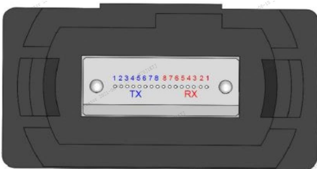
Figure 7.2 MPO-16 Optical Connector Interface
