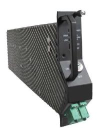
along with the 14 slot OTC chassis. The Luxglo EDFA module houses one complete independently managed optical amplifier in a single slot wide case allowing a single Luxglo OTC chassis to support up to 14 distribution networks in a small 4RU head-end equipment space. This hot swappable module features front panel key switch, diagnostics and supports SNMP for remote monitoring.
